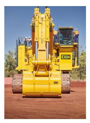
The new excavator will be operating around the clock at the Callide Mine, put to work for more than 400 hours each month and expected to shift 5.0 million bcms of waste each year.
