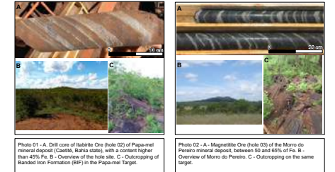
Photo 01 - A. Drill core of labirite Ore (hole 02) of Papa-mel mineral deposit (Caetité, Bahia state), with a content higher than 65% Fe. B. Overview of the hole site. C. Outcropping of Banded Iron Formation (BIF) in the Papa-mel Target.
