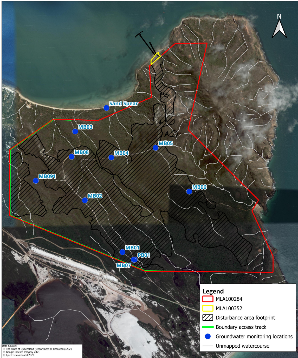
Cape Flattery Silica Pty Ltd Cape Flattery Silica Sand Project Initial Advice Statement Figure 15 Groundwater monitoring locations Scale: 1:20,000 Datum: GDA 2020 Projection: MGA zone 55
