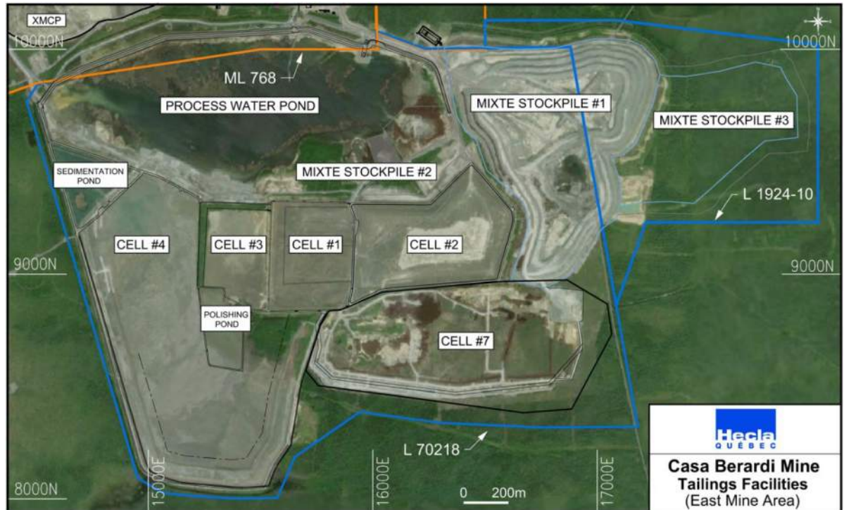
Figure 15-4. Surface Plan Tailings and Waste Rock Facilities
