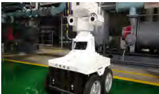
Beijing Gas-fired Power Plant's intelligent inspection robot
