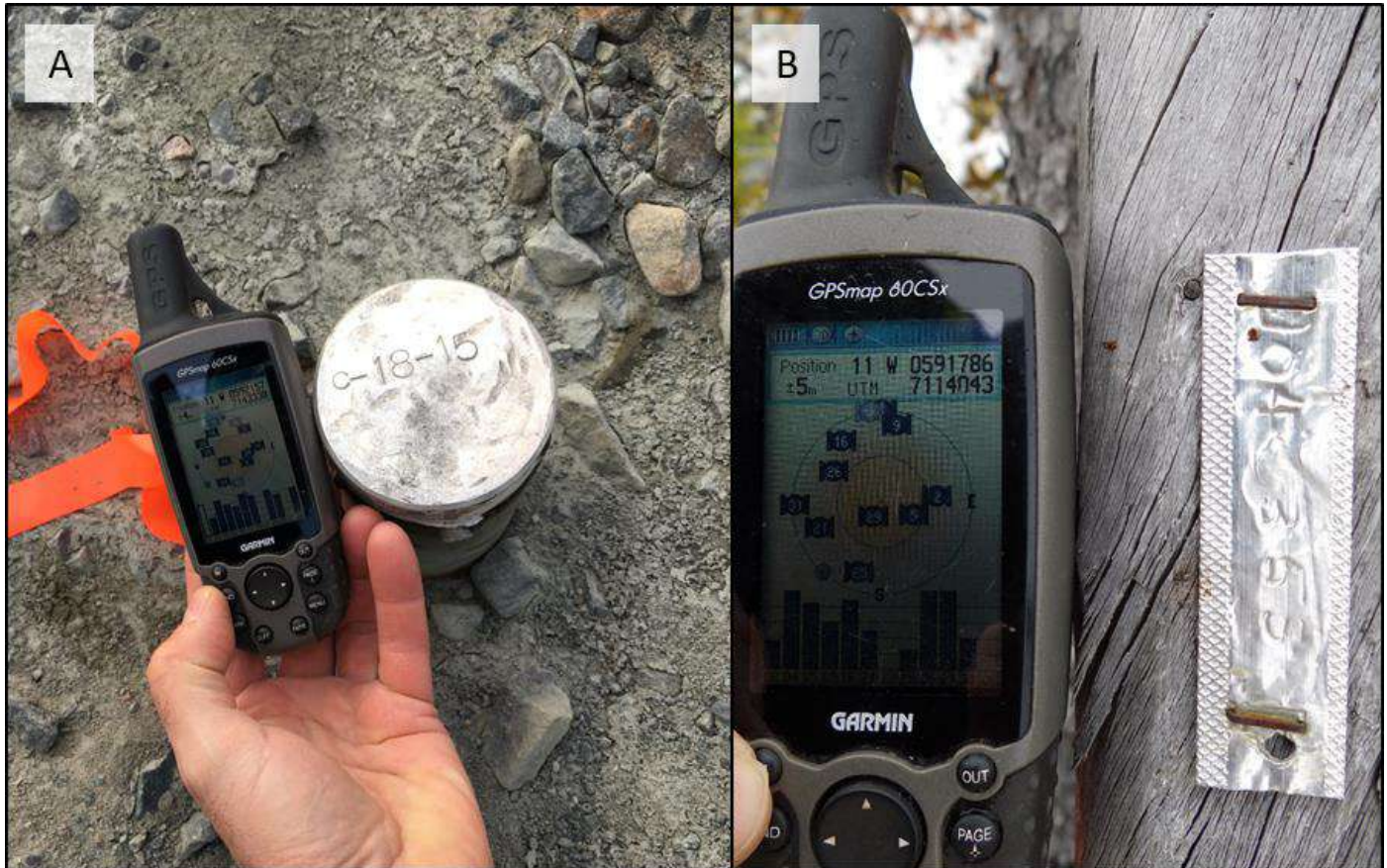
Figure 12-2: Examples of On-Site Collar Location Verifications
