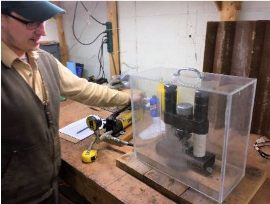
Figure 10.6: Point Load Testing (Bemek Rock Tester)
