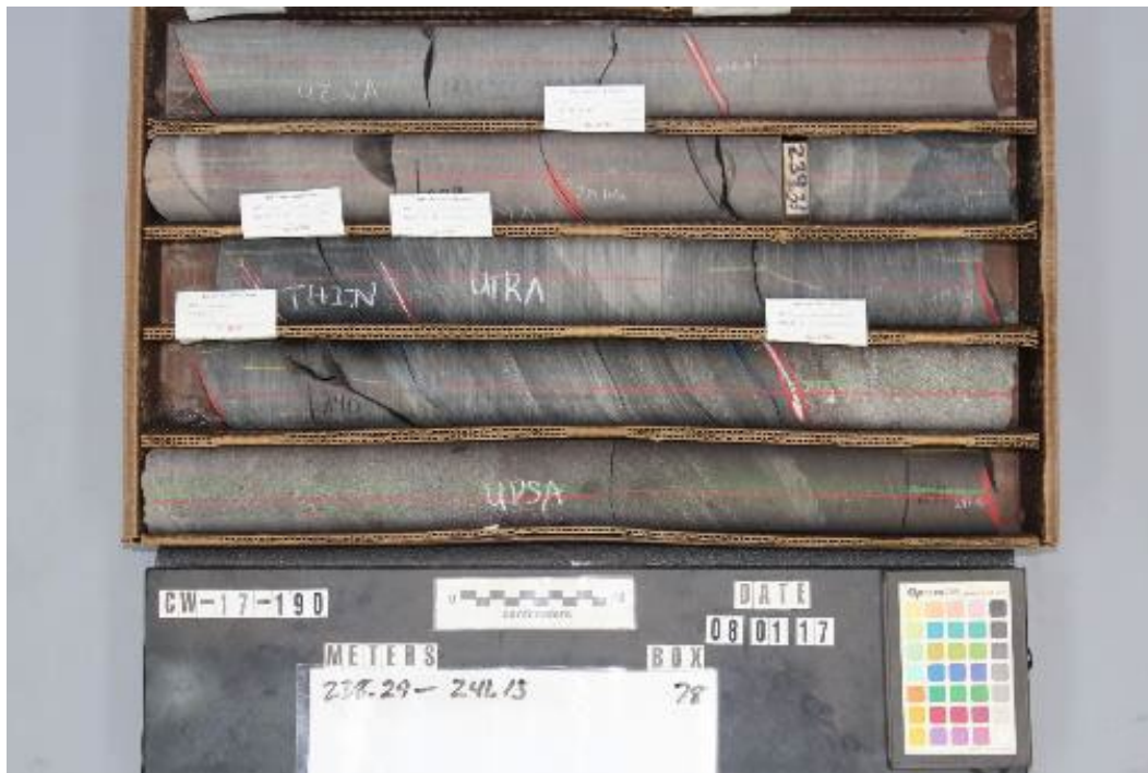
Figure 10.10: Bottom of UCBS Showing Marked Intervals for Assay Sampling
