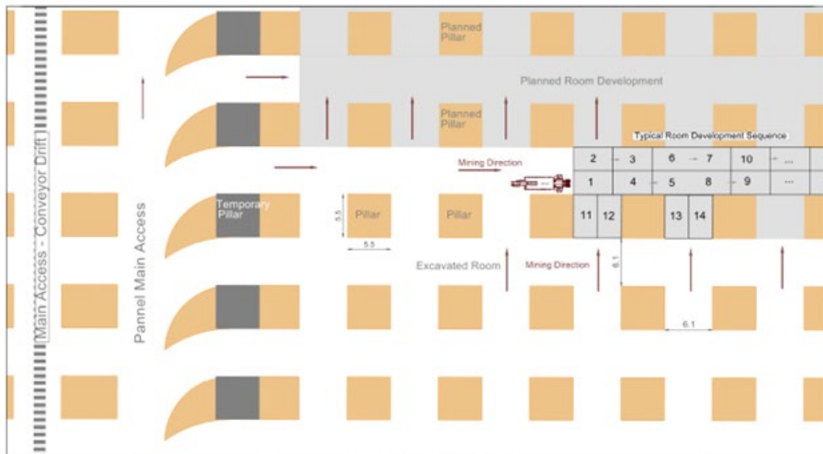
Figure 1.4: Continuous Miner Room Development Sequence
