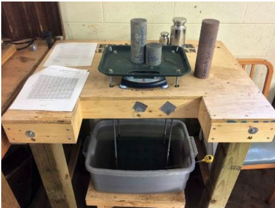
Figure 10.7: Specific Gravity Station
