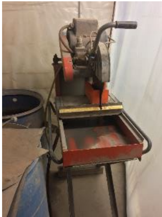
Figure 10.3: Core Saw Station at White Pine Site
