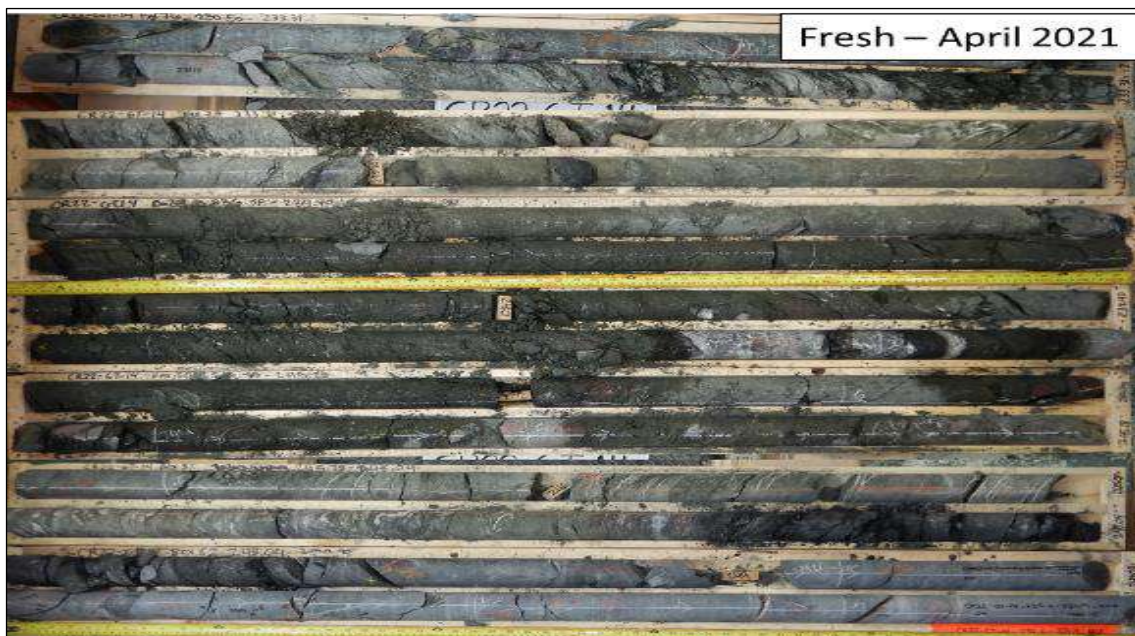
Figure 16-7: Example Image of Drill Core from the Modelled CUC Fault Core and Damage Zone
