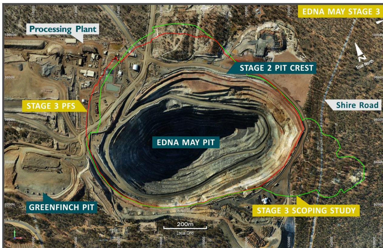
Figure 1: Edna May Plan view – existing pits, Stage 3 Scoping Study & PFS pit outlines
