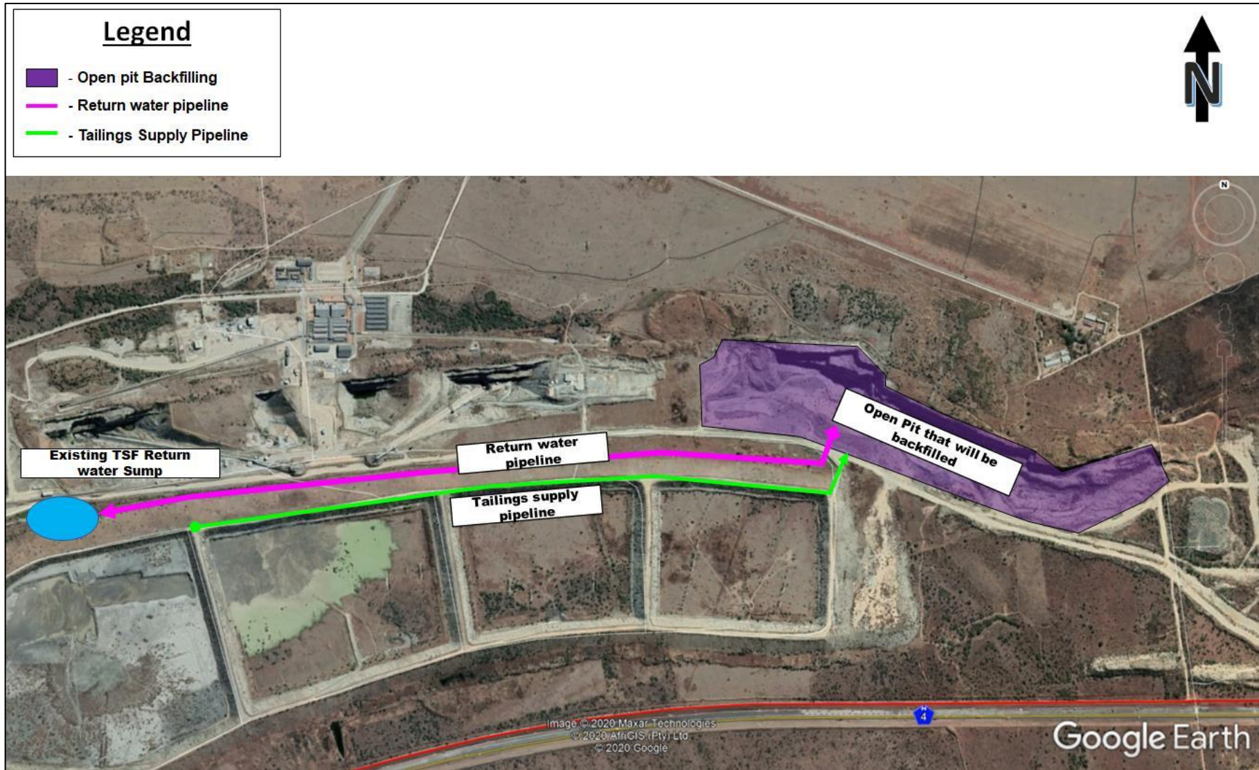
Figure 8: Aerial Map of the Opencast Pits Backfilling Project, including associated infrastructure.
