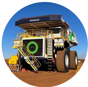
Battery electric truck with Liebherr/WAE
