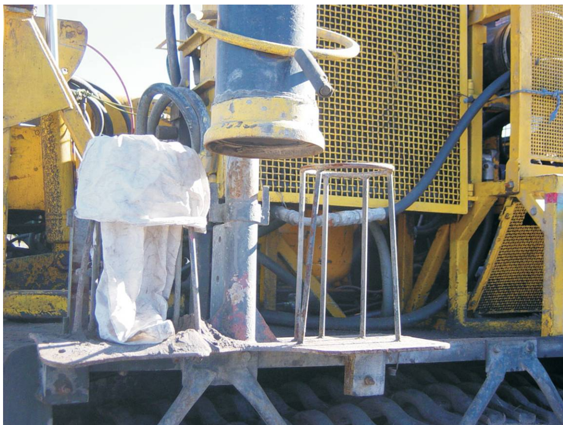
Figure 11.1 RC Sample Collection Cyclone and Sample Bag – MDL Drill Rig No 1
