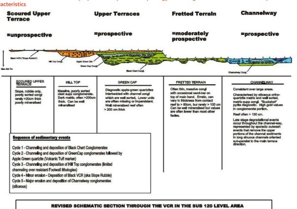
REVISED SCHEMATIC SECTION THROUGH THE MPONENG MINE INTRODUCTION
