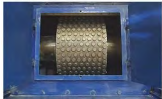
Figure 13-11. View of SMALLWAL HPGR unit at KCA Used for Testing Hasbrouck Mine Samples
