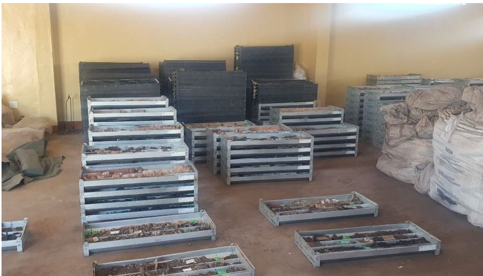
Figure 12.4 Core processing facility showing stacking and storage of core trays; core trays in foreground laid out for Qualified Person inspection
