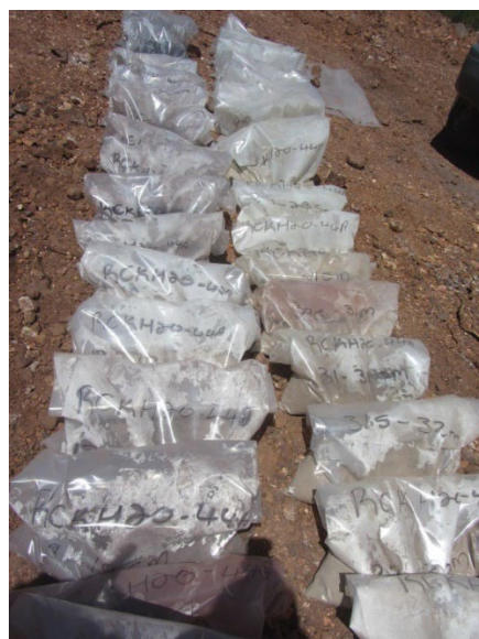
Figure 10.6 RC samples laid out sequentially at the rig
