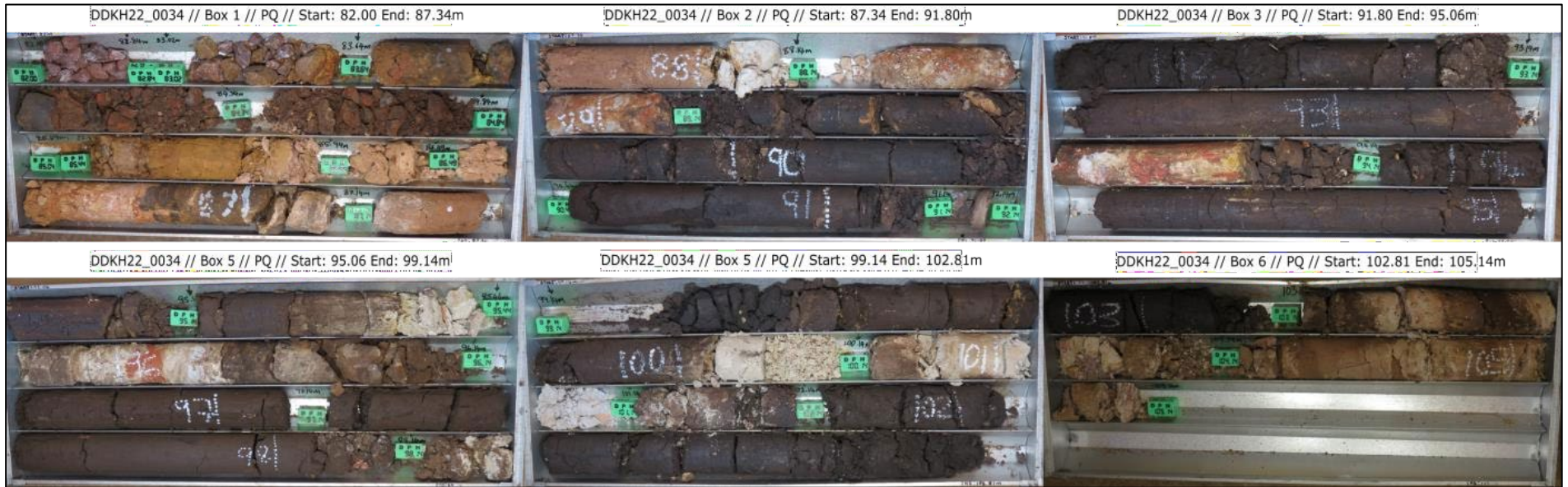
Figure 10.3 An example of completed photograph collage of a diamond drillhole at the K.Hill Project
