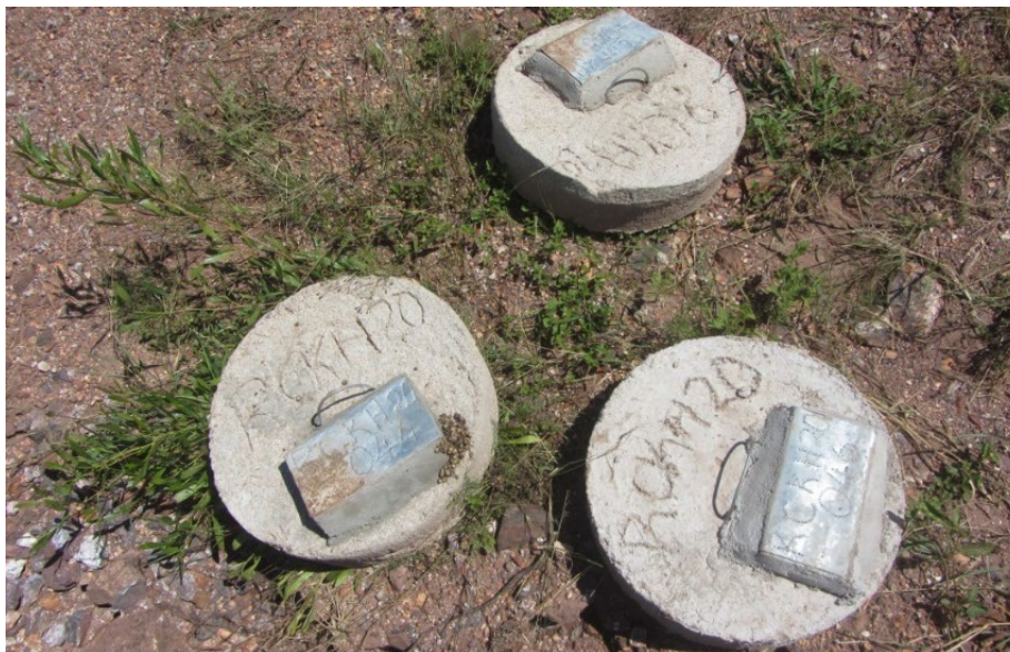
Figure 10.4 Concrete reverse circulation collar plugs used to close and mark completed reverse circulation holes
