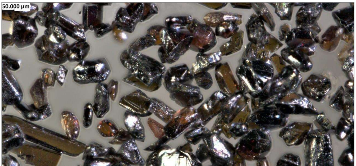
Figure 25: Photomicrograph of high purity rutile product
