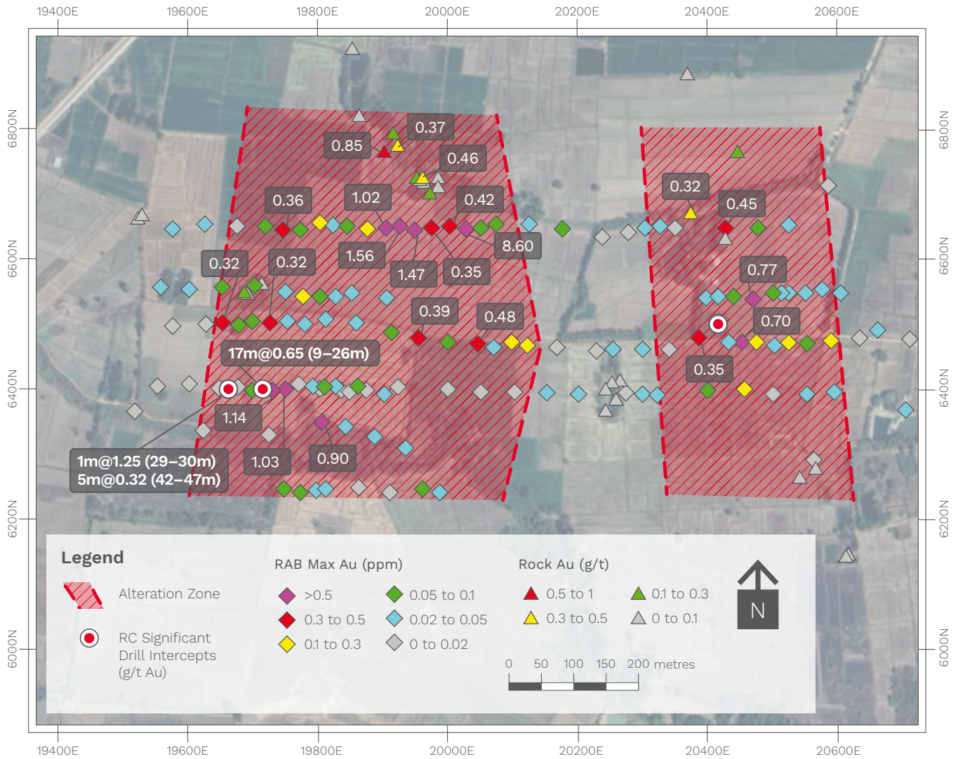
Figure 7: Map showing alteration zone (red hatching) in Jorakae Prospect, rock, RAB max Au and RC assay highlight
