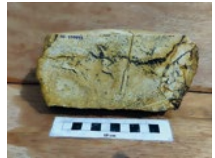
^ Figure 6: Rock slab of silicified rock with 0.85 g/t Au (RF530392) and silicified rhyolitic tuff with 0.37 g/t Au (RF530393) in Jorakae Prospect
