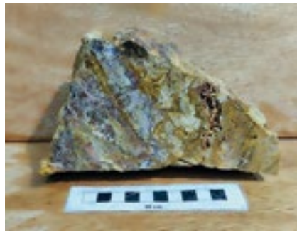
^ Figure 6: Rock slab of silicified rock with 0.85 g/t Au (RF530392) and silicified rhyolitic tuff with 0.37 g/t Au (RF530393) in Jorakae Prospect
