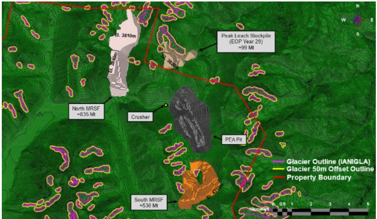
Figure 16.34: Location of Mine Rock Storage Facilities and Leach Stockpile for 125 ktpa Alternative Case
