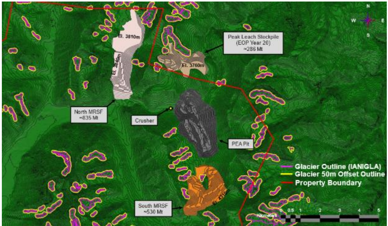
Figure 16.33: Location of Mine Rock Storage Facilities and Leach Stockpile for 175 ktpa Base Case
