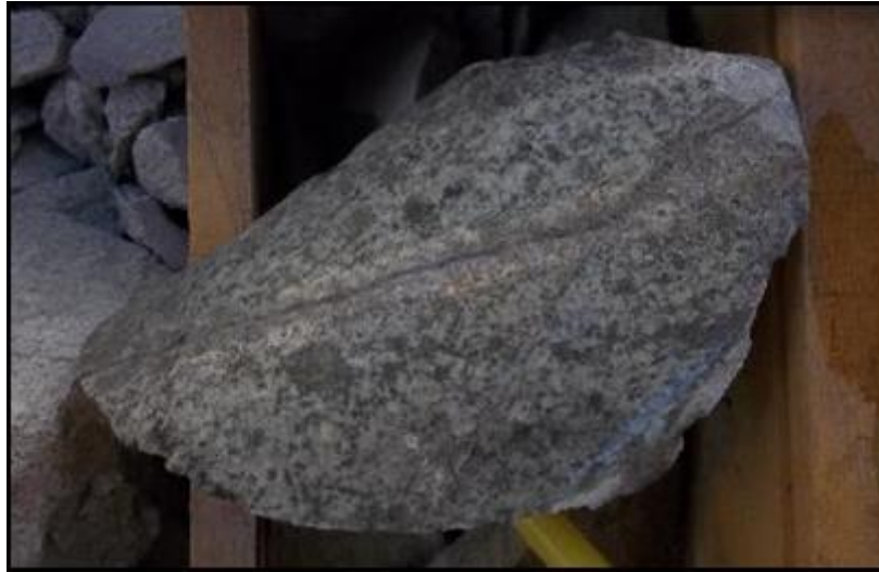
Figure 7.8: Equigranular diorite (pre-mineral pluton) with chlorite alteration cut by a hairline type- D veinlet containing quartz and chalcopyrite with a sericite alteration halo (Hole AZ1284, 173 m).
