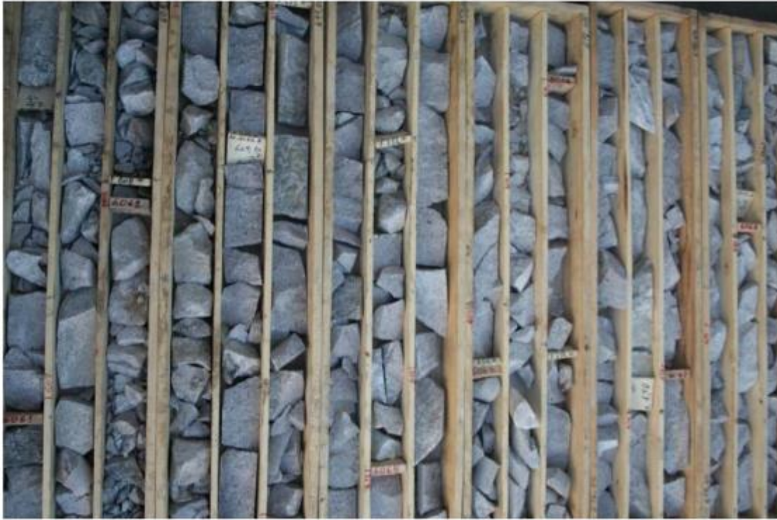
Figure 7.18: Typical Drill Core from Los Azules indicating the strongly fractured nature of the rock (Jemielita, 2010)
