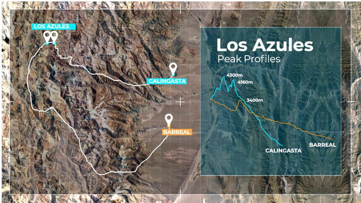
Figure 18.4: Site Access Road Profiles (McEwen)
