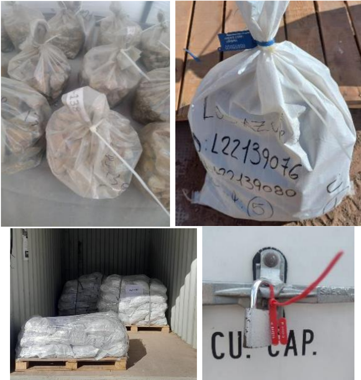
Figure 11.5: Showing the sequence of bagging, tagging, sealing, and securing the samples for dispatch
