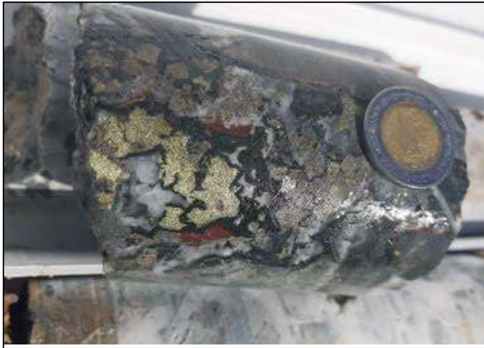
FIGURE 7.6 PHOTOGRAPH OF DRILL CORE SHOWING SULPHIDE MINERALS
