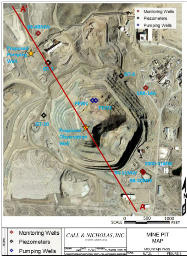
Figure 13-10: Location of Proposed Pumping and Monitoring Wells by CNI Shown in Plan-View
