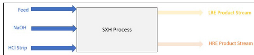
Figure 10-9: Diagram of the SXH Process
