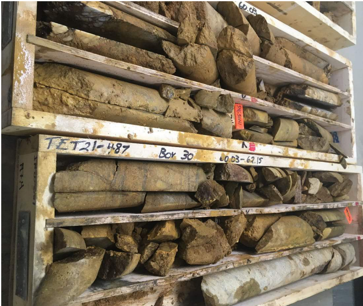
FIGURE 7-9 EXAMPLE OF SPLIT CORE PRIOR TO SAMPLING, TETLIN PROJECT, ALASKA
