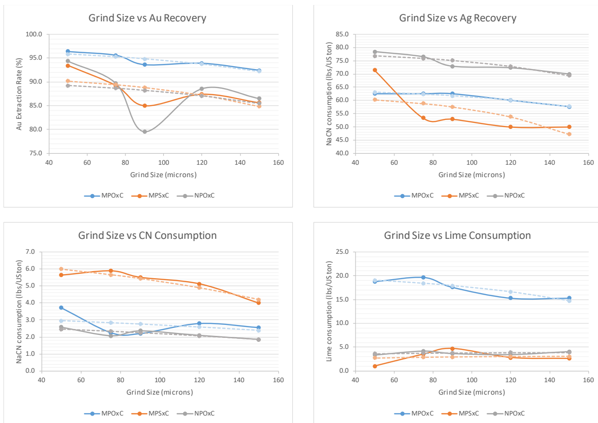
FIGURE 10-22 LEACH GRIND SIZE OPTIMIZATION
