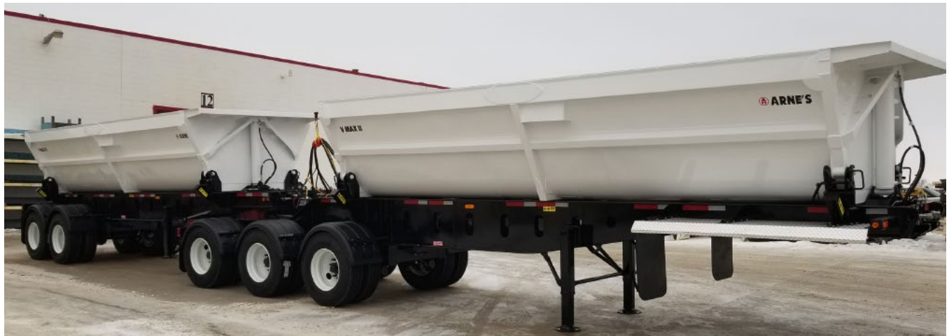
Figure 18.7: Example of Dual-trailer Side-dump Trailer with a Max 36-40 t Capacity
