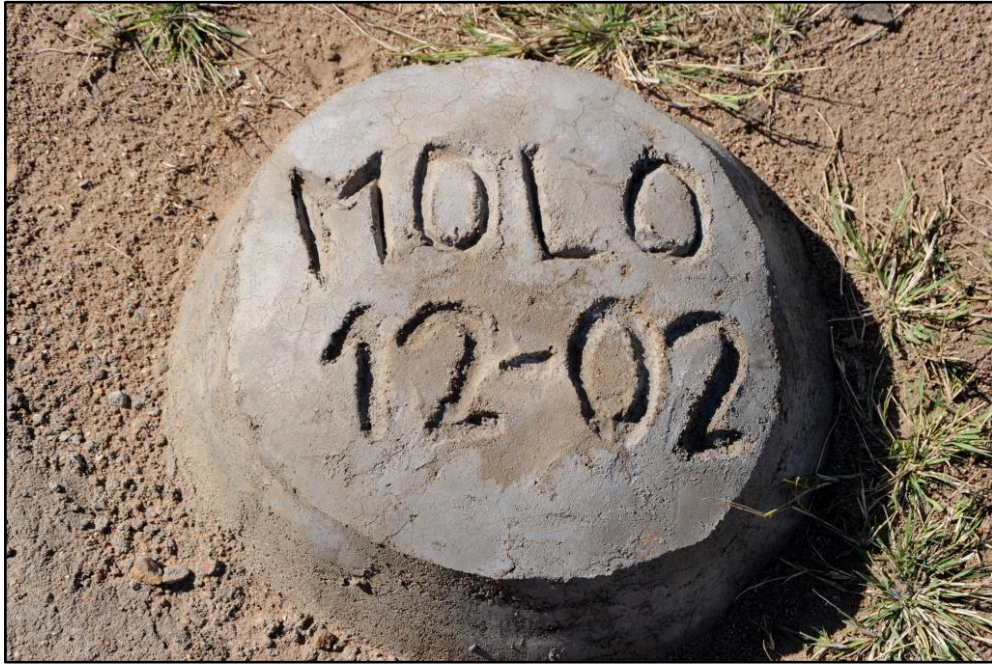
Photo 6: Concrete Marker Showing the Collar Position of Borehole Molo 12-02 (as Supplied to CCIC by the Company )
