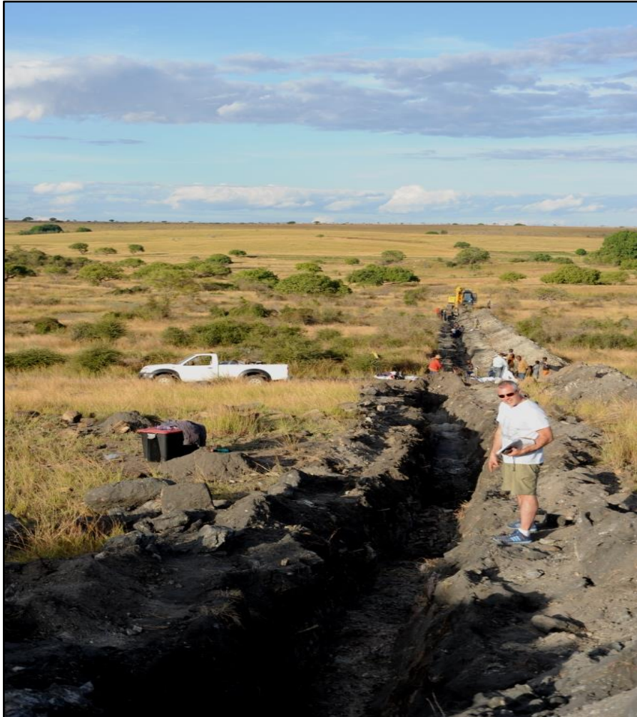
Photo 4: Trenching for the Bulk Sample on Molo, May 2013
