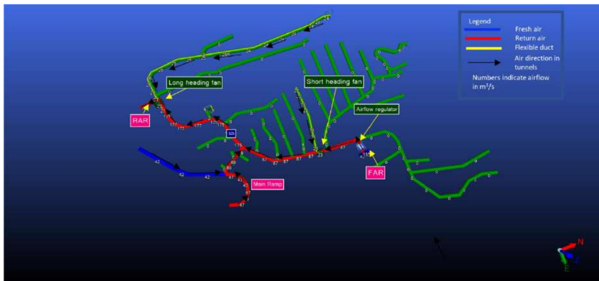
Figure 16.15 – Auxiliary Ventilation Production Level
