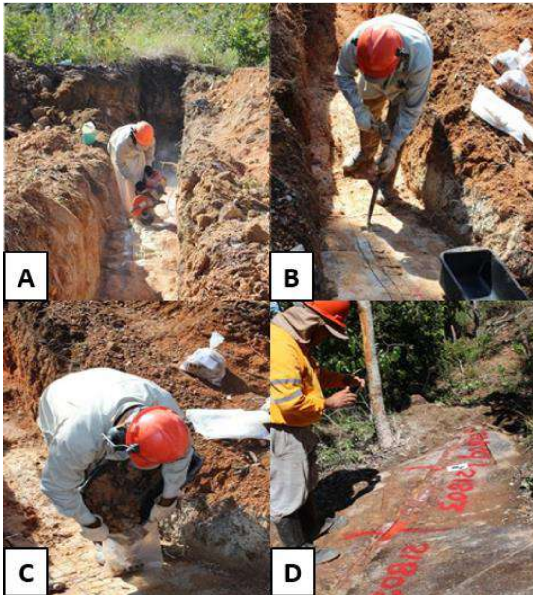
(A and B) Channel samples collection; (C) 1 m samples stored in plastic bags; (d) 1 m channel after sampling.
