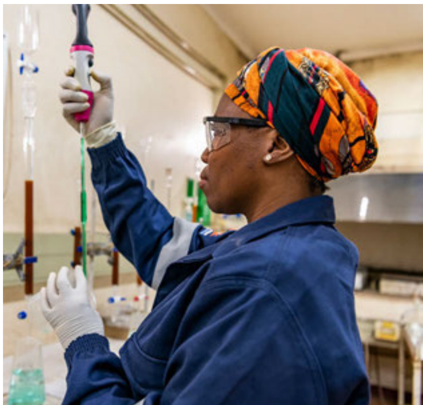
Titration in the wet chemistry section of the Zondereinde assay laboratory
