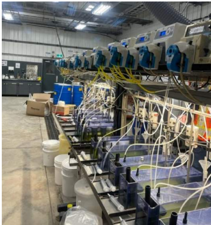
Figure 13-5: Continuous SX Mini Pilot Test Set-Up
