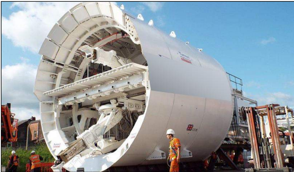
Figure 16-8: Typical Tunnel Shield Equipment Setup for Soft Ground Excavation
