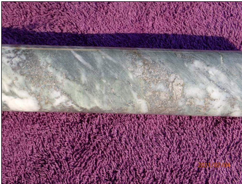
Figure 7-22: North Zone Vein and Alteration Characteristic
