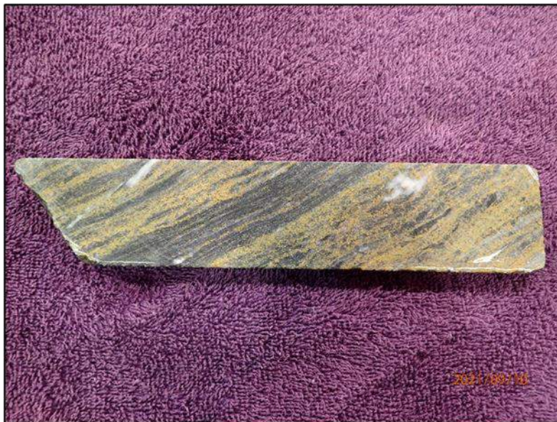
Figure 7-16: Banded Sphalerite – Black Silica RR28Z
