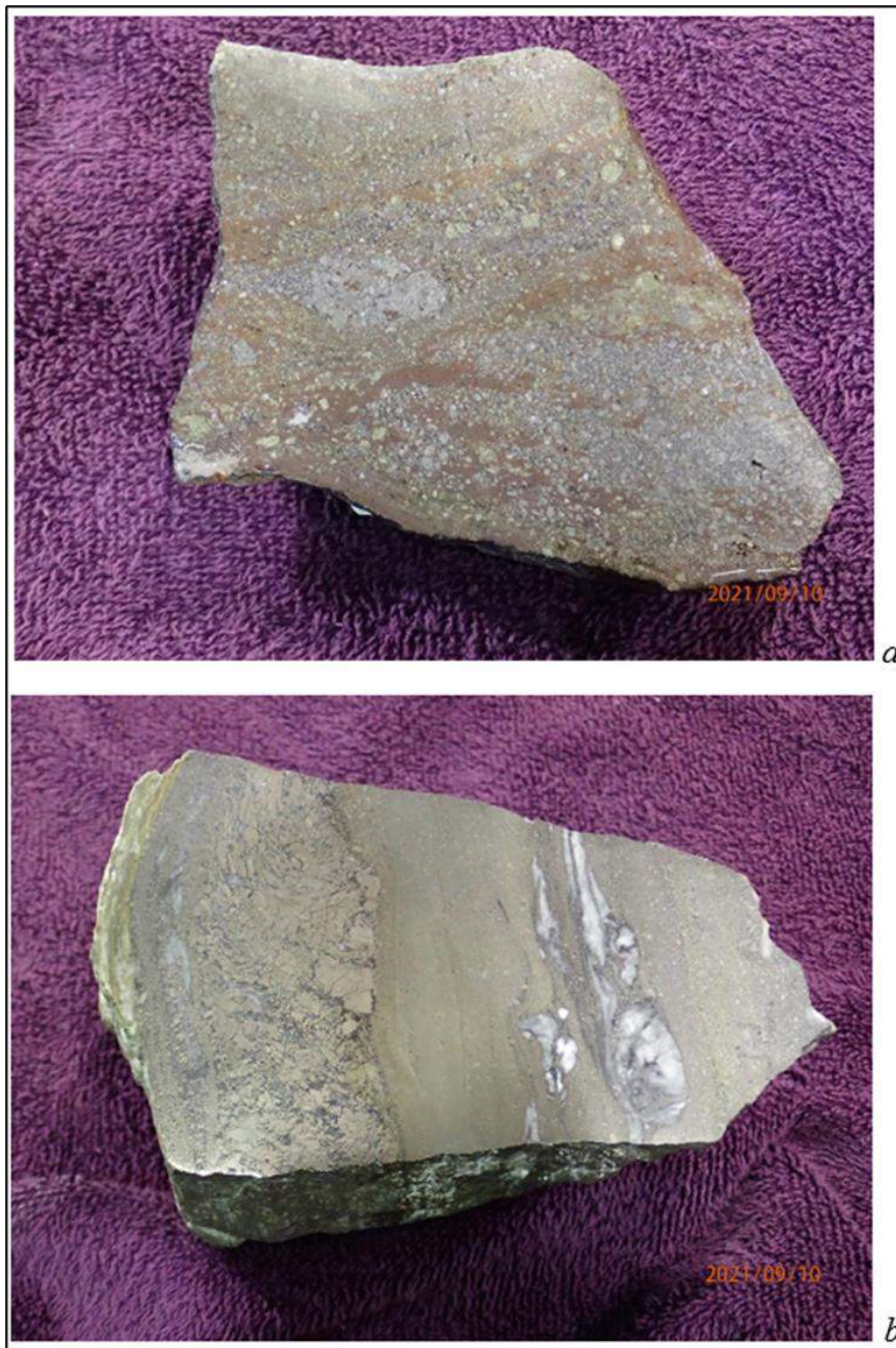
Figure 7-13: Textural Characteristics RRMZ Sulphide Bands
