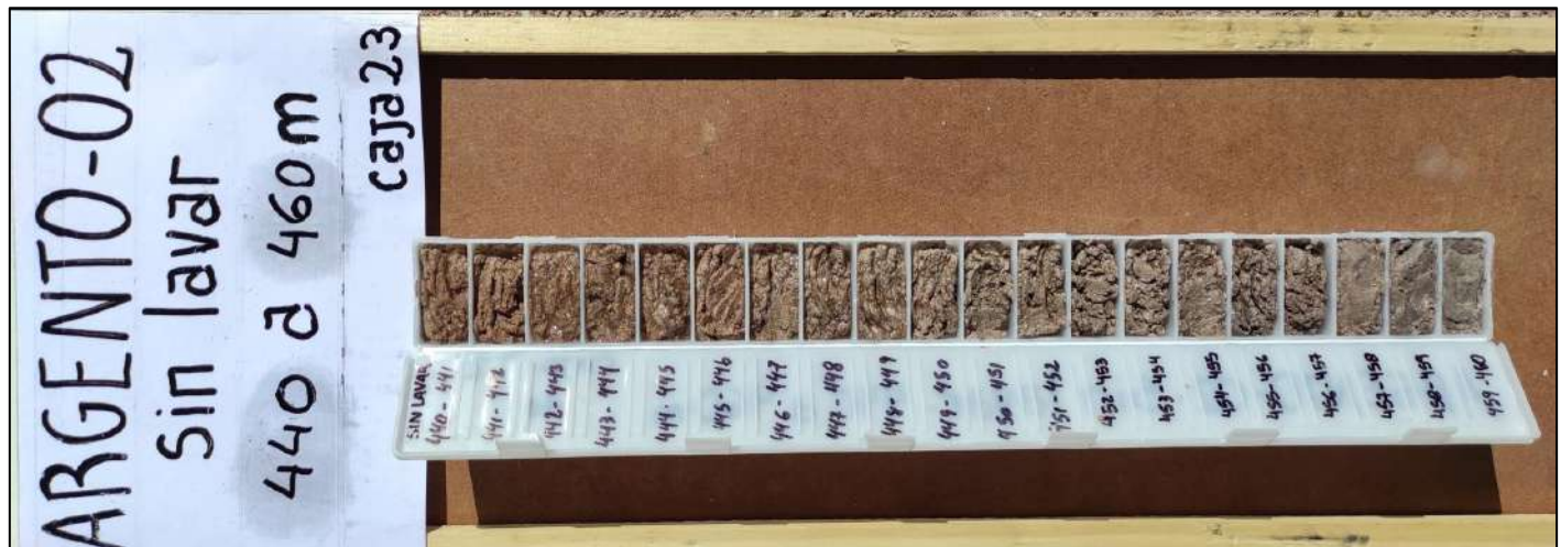
Figure 10-10: Example of Drill Cuttings From Exploration Well Argento-02
