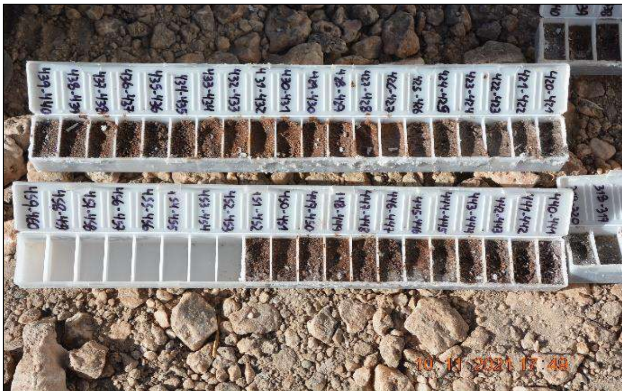
Figure 10-2: Example of Drill Cuttings From Exploration Well Argento-01
