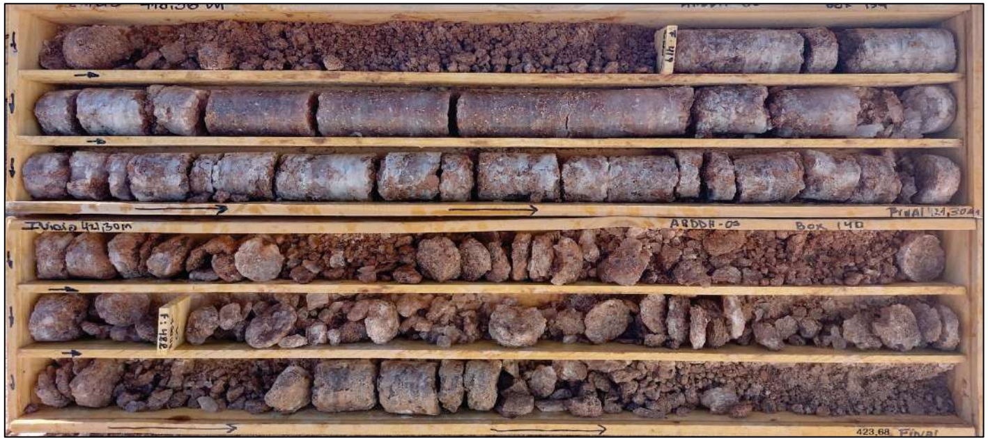
Figure 10-27: Core Samples Obtained During Drilling of Borehole ARDDH-05
