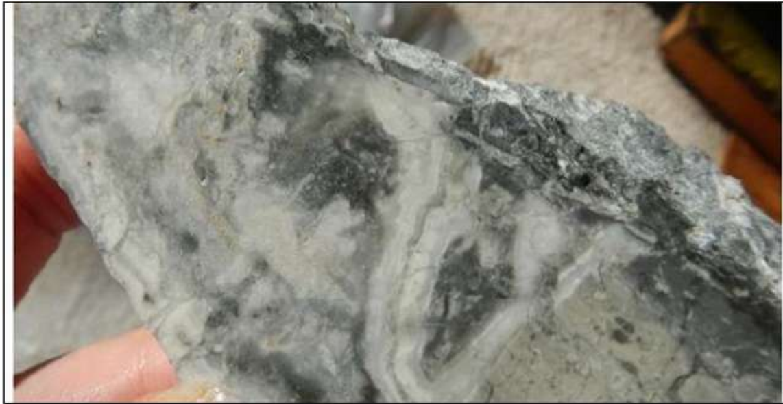
FIGURE 7.12 VEIN ZONE 2A IN DRILL HOLE SN18-18 (AT 285.8 M)
