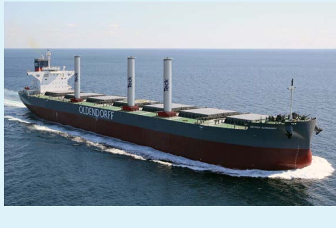
Picture: A rendering of the Oldendorff ship outfitted with a Flettner Rotor system.
