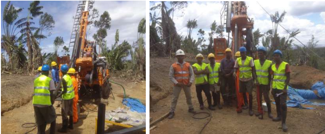
Fig.: Company owned diamond core drilling machine in operation during exploration 2018-19
