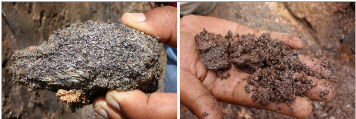
Figure 3-9: Jumbo flakes of graphite (Left); Small flakes of graphite (Right) as observed in Sahamamy and Vatomina sites
