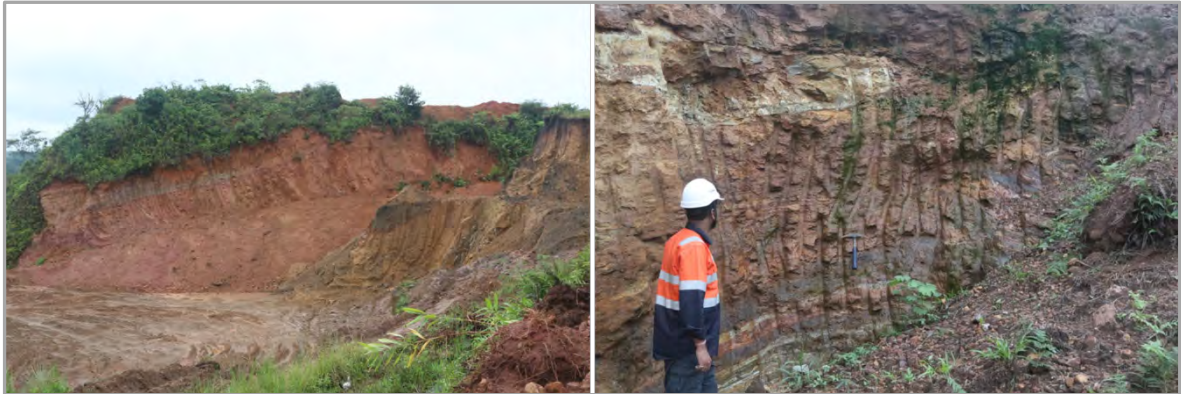
Figure 3-7: Graphite mineralisation within the saprolite (Left); Contact between 'High' grade and 'Medium' grade graphite ore body (Right) as observed in Sahamamy project
