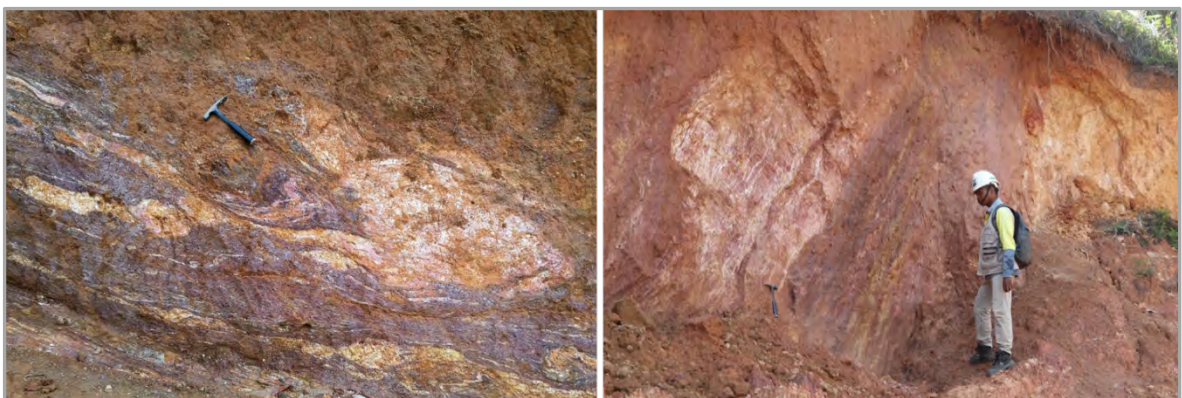
Figure 3-11: Early F1|F2 Folds of graphitic zones (dark colour) within Khondalite (Left); Steeply dipping graphitic zones (Right), as observed in Vatomina site
