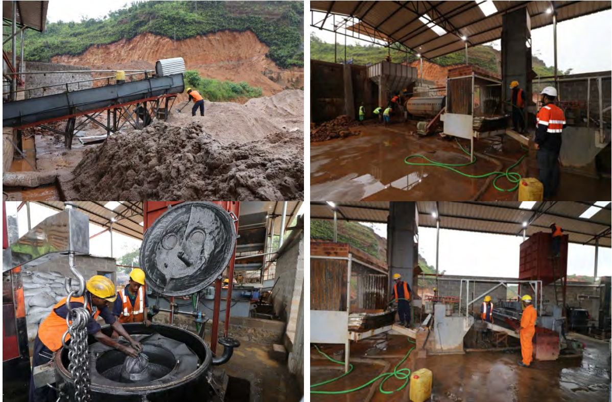
Figure 7-4: Process plant photograph taken during plant site visit in June 2019; hopper, ball mill, scrubber-classifier SAGE, ball mill discharge point, centrifuge recovery of graphite
