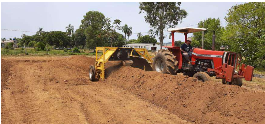
Figure 17: Prototype of windrow turner in operation
