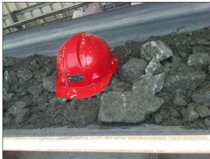
Figure 10-Ore on mill feed conveyor (helmet as scale)
