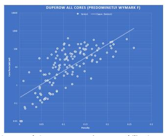
Figure 14.3: Wymark Core Data: Porosity Permeability Cross-Plot
