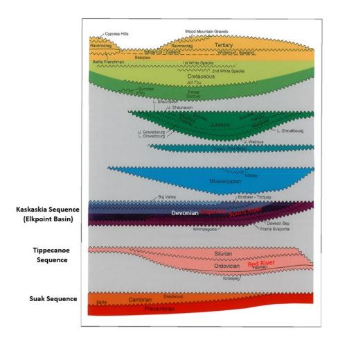
Figure 7.1: Williston Basin deposition with representative unconformities and thickness (modified from Kent 92)
