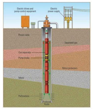
Figure 16.3: Typical Electric Submersible Pump Configuration
