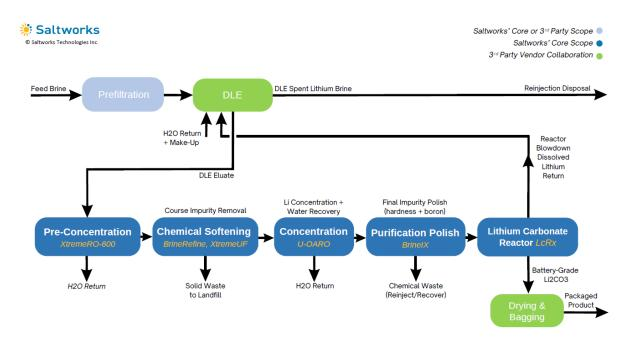
Figure 17.1: Schematic of Proposed DLE and CRC Process
