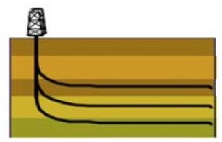
Figure 16.2: Multi-Leg (Stacked) Well Schematic
