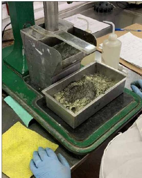
Figure 13.20: Final Concentrate Containing Copper and Molybdenum
