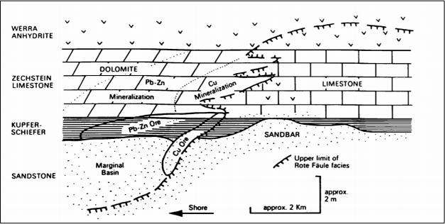
Figure 8.2: Schematic Cross-section Showing the Position of Rote Fäule in Relation to Lithological Types and Mineralization
