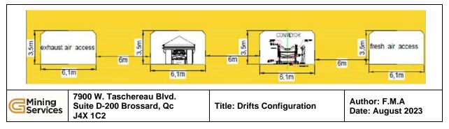
All drifts are set at a 6.1 m width, and their height varies from a minimum of 3.5 m to a maximum of 6.1 m. Most of the development will be performed by continuous miners. Continuous miners require a minimum opening of 3.5 m and can mine up to 5.8 m. Anything higher than 5.8 m would be mined with jumbos.
