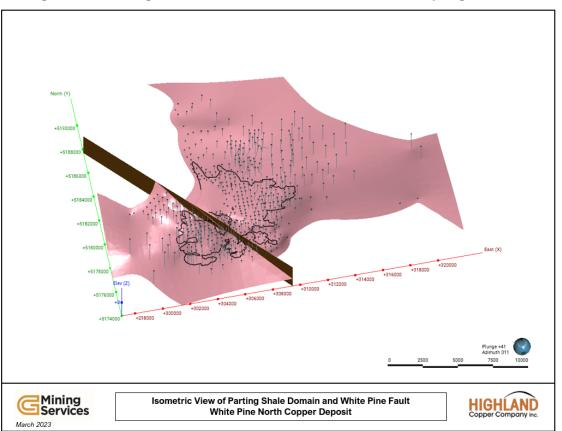
Figure 14.4: Parting Shale Wireframe and White Pine Fault—Leapfrog 3D Model
