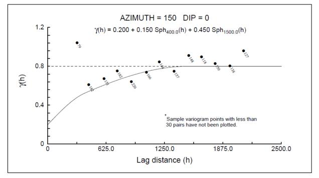
Figure 14.13: Variogram Model Cu% for the Parting Shale (PS) Column
