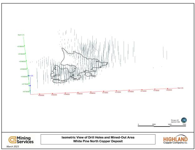
Figure 14.2: 3D View of Drill Holes and Mined-Out Area, View Towards Northeast
