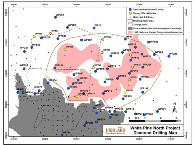
Figure 9.1: Location Map of Holes Completed During 2014 Drilling Program and Historical Diamond Drill Holes Used in WPC's Validation Sampling Program
