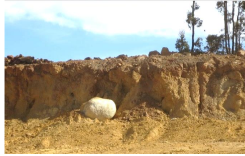
Hardcap (hard brown) Friable (soft yellow), relict fresh remnant Dolerite dyke boulder
