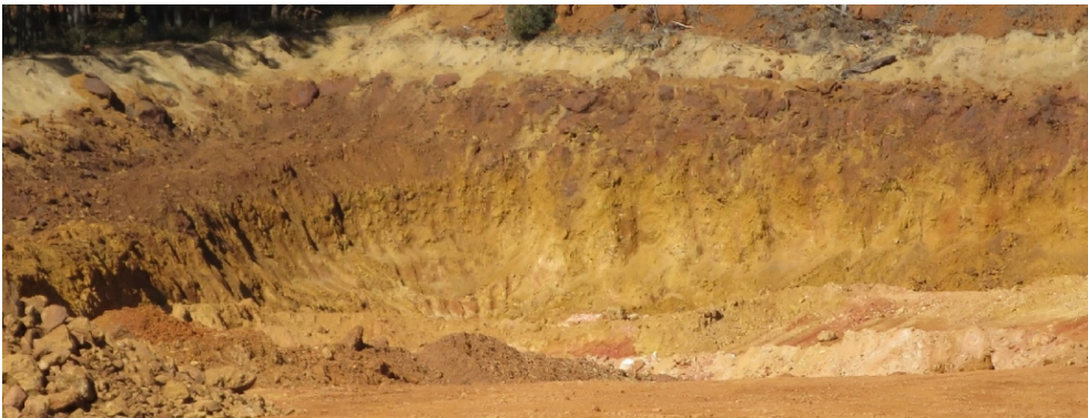
Sandy topsoil, Hardcap (hard brown), Friable (soft yellow), Basal Clay (white clay, lower right in the floor).
