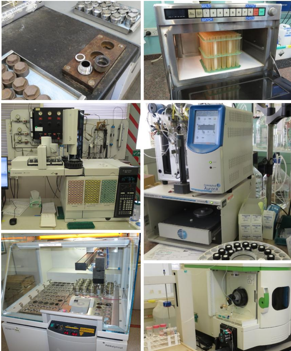
Figure 8-6: Digestion and Assay Equipment used for REF Samples at the KWI Clockwise from top left: BD, MD, TICTOC, ICP, XRF, GC (SLR, 2021)
