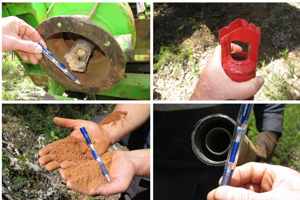
Figure 7-3: Drill Bits, Reverse Circulation Drill String and Particle Size of the Sample Residue (SLR, 2021)
