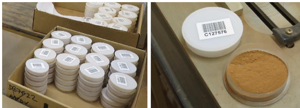
Figure 8-2: The Pulverized Sample is Stored in a Barcoded Dedicated Receptacle for Assay (SLR, 2021)
