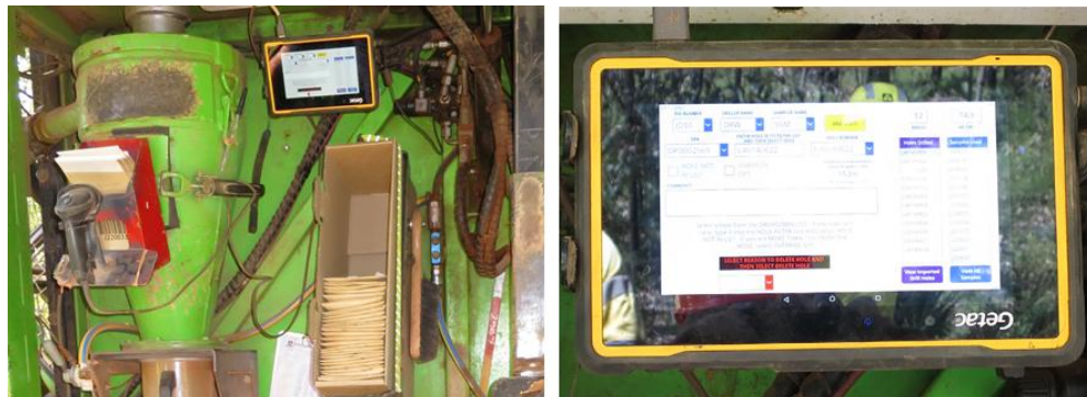
Figure 7-5: Barcode Reader and Digital Recorder Mounted on the Drill Rig (SLR, 2021)
