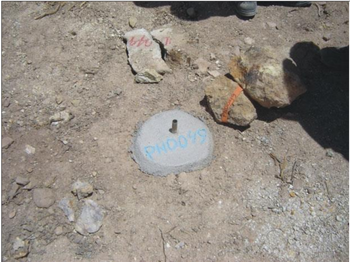
Figure 10-6: Example of Drill Collar Cap
