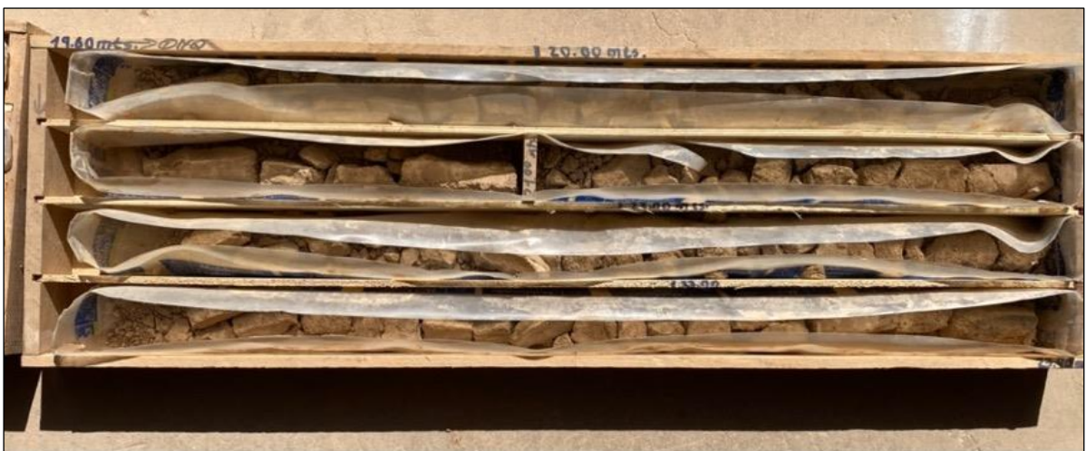
Figure 10-3: Typical Sonic Core Samples
