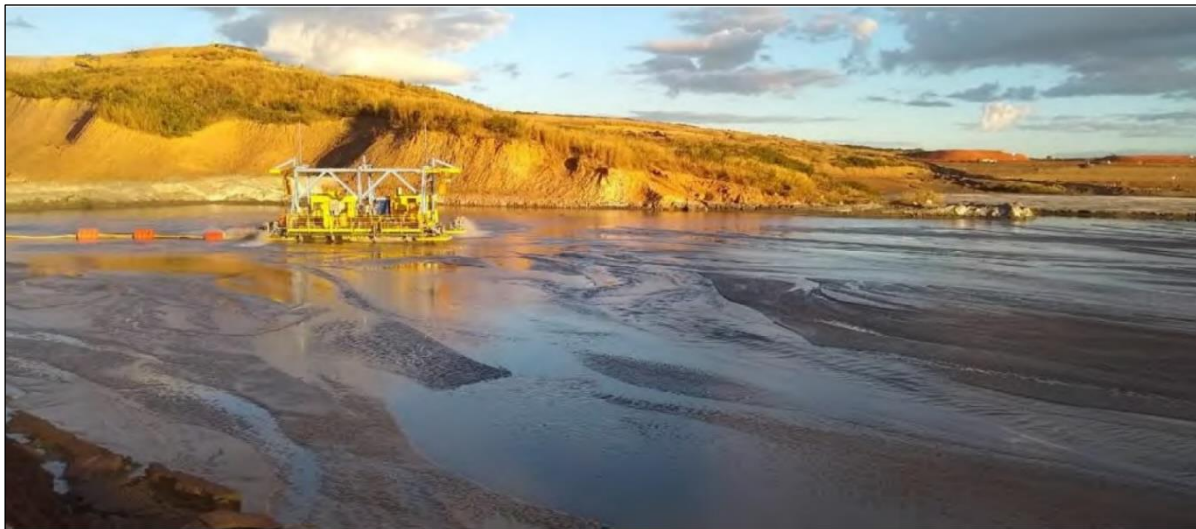
Figure 16-3: Dredging Pontoon with Submersible Pumps
