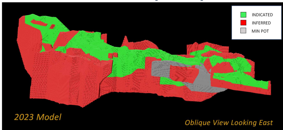
Figure 14-28 Larkin Mineral Resource Classification - long section looking east
