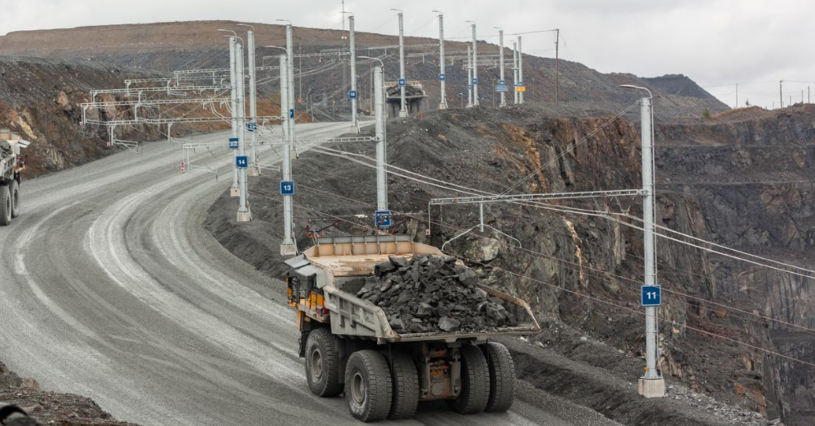
Electrified ore haulage at Boliden Kevitsa.
