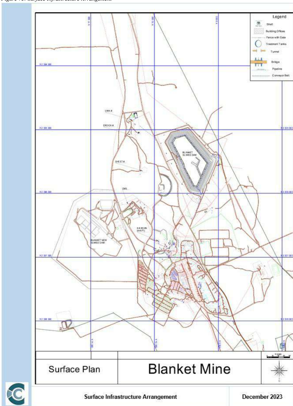
Figure 73: Surface Infrastructure Arrangement
