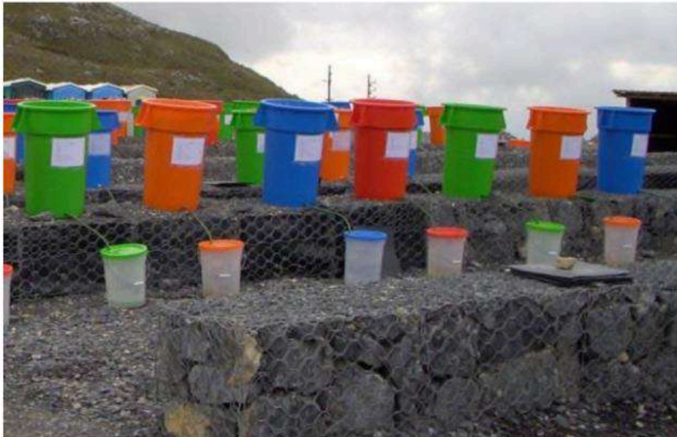
Figure 10.3.2: Environmental aging barrel tests
