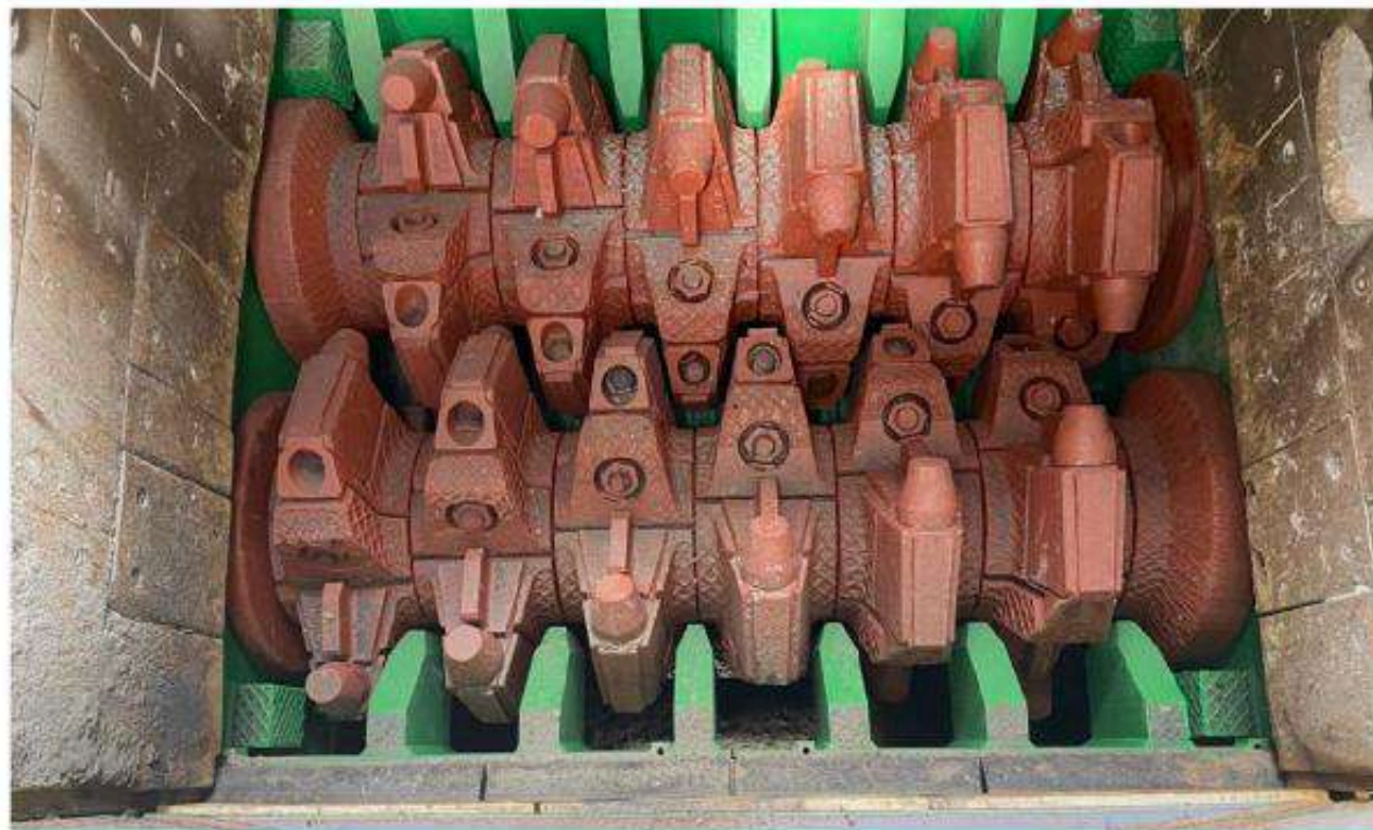
Figure 14.1.2: Crushing chamber of new primary crusher (MMD Sizer) installed at Cerro Corona in 2022
