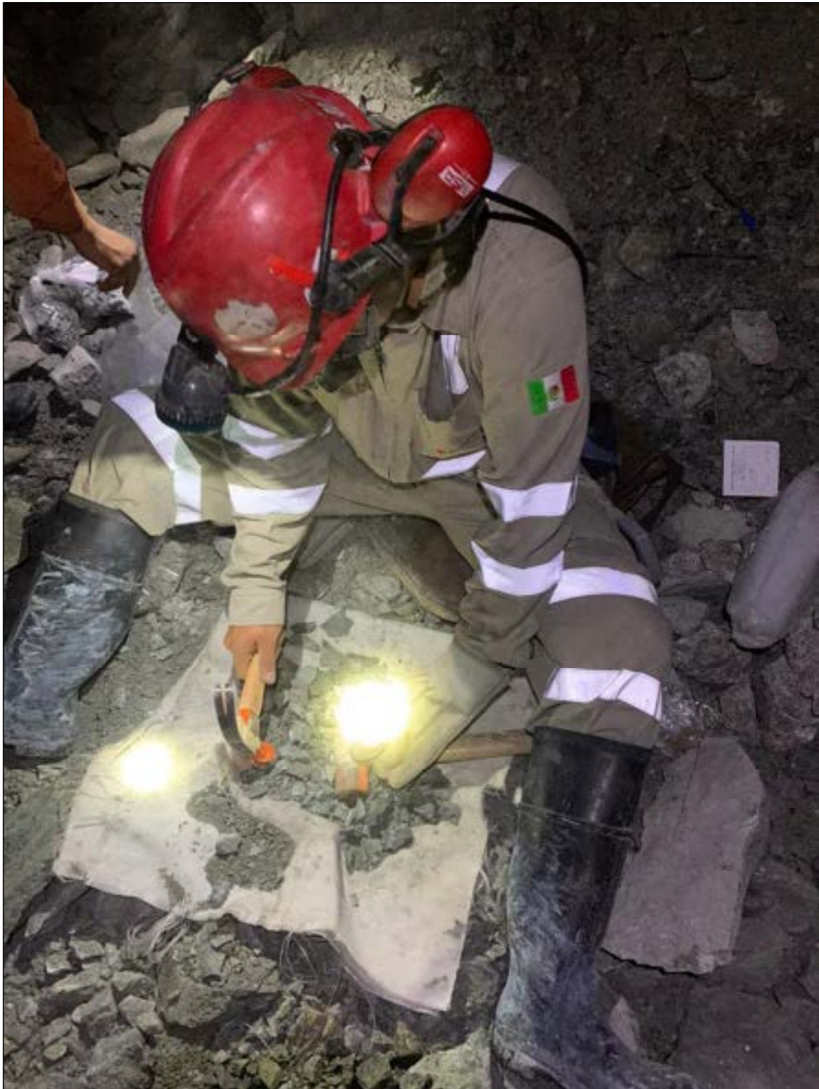
Figure 7-5: Homogenization Process of Sample Particle Size
