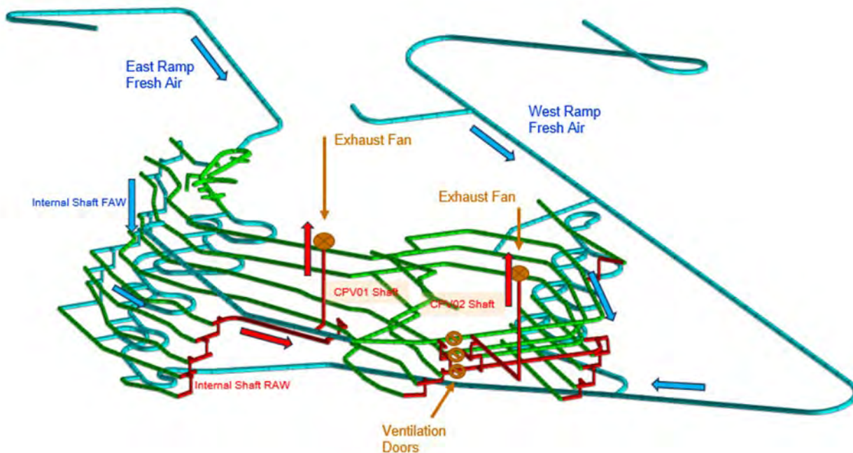
Figure 1-5 Isometric view of the Main Ventilation Network from the NW
