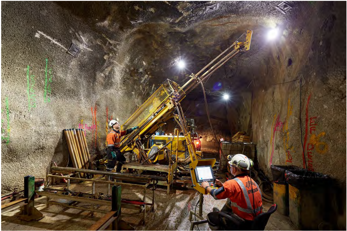
Figure 10-3: Diamond Drill Rig in an Underground Drill Station
