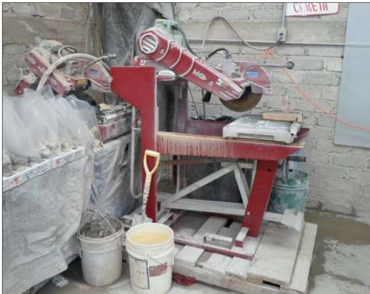
Figure 11.2. One of several core saws located at the exploration core facility Source: VanGold, 2018
