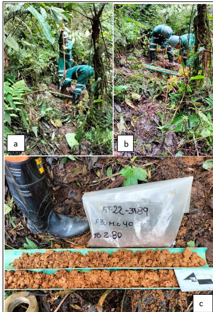
Figure 9.11 Soil sampling process: a) Location of the auger in the mesh; b) Insertion of the auger into the soil layer; c) Extraction of the soil sample and its coding for sending to the laboratory.
