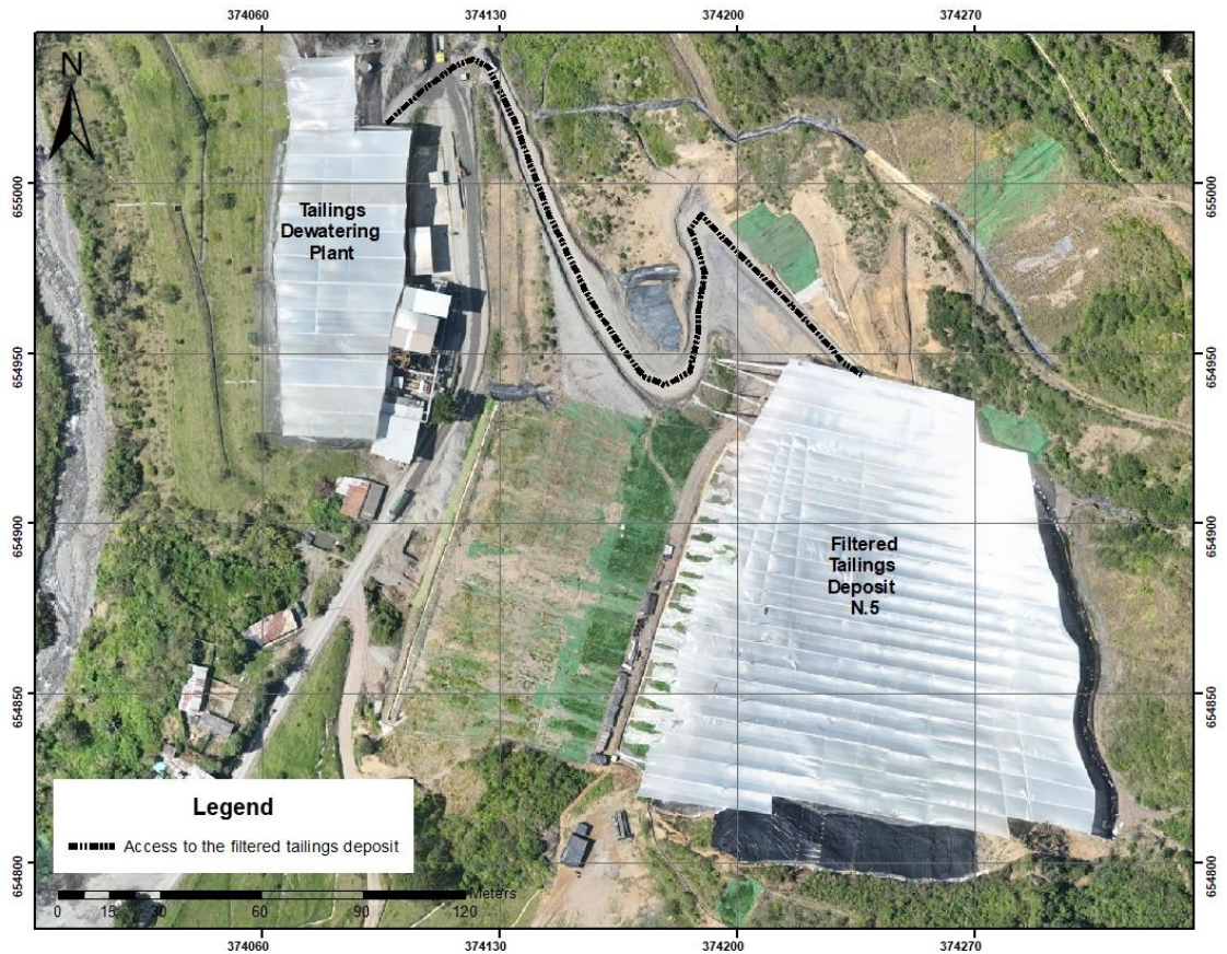
Figure 18.2 Dewatering plant and dry filtered Tailings Deposit Numero 5.
