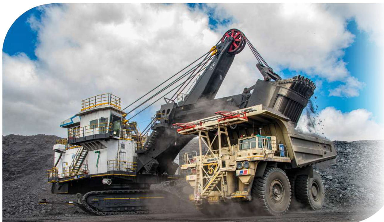
Rope shovel loading coal at Grootegeluk
