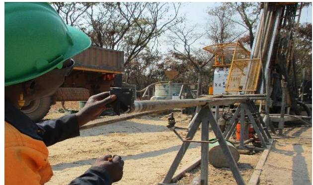
Figure K6: Oriented diamond drilling campaign at Kagem.
