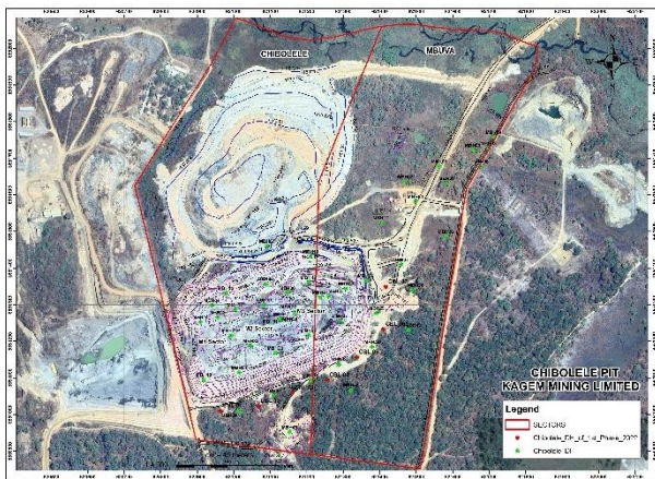
Figure K8: Chibolele Pit-Shell and collar locations
